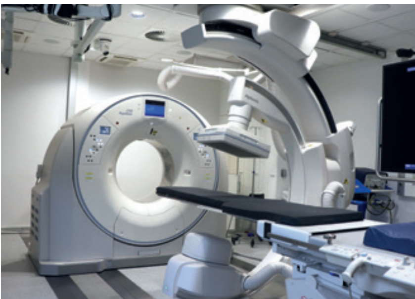
Canon's Alphenix 4D CT installed in the Department of Radiology, UZ Brussels, Belgium.
