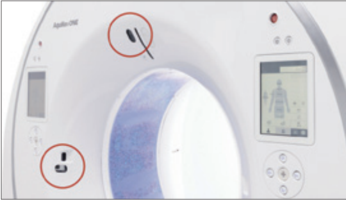
Figure 2: Dual gantry mounted cameras.
